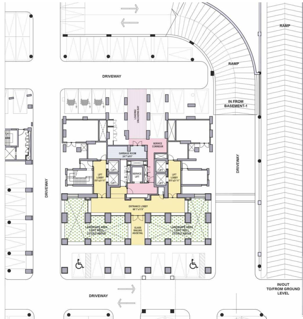
The Service Ramp is directly connected to the lower basement with loading/unloading docks for each tower. These service entrances from the loading dock connect to the service lobby and the service elevator. There is a garbage chute on each floor with collection room in lower basement.
